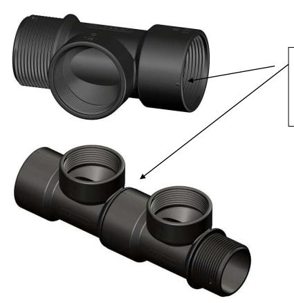
Align the two location notches. There is no need to tighten fully. When adhesive type thread sealant is used, fittings need only be "finger tight" as the sealant will provide full waterproofness and structure once cured. This allows the two fittings to align.
