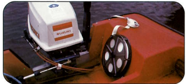
Another mounting on a boat with a motorwell. The anchor can be stored under the motor. The webbing can also be made fast to the bow cleat.
