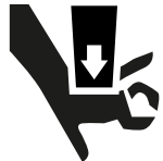
Caution: risk of crushing
