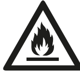
Attention: fire hazard
